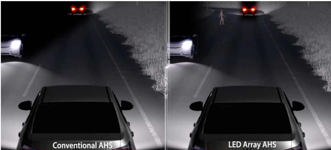
Figure 12. Toyotas conventional AHS system has poor illumination of adjacent areas and is not able to illuminate the pedestrian crossing the road behind the oncoming care. The LED Array AHS allows for a greater illumination of surrounding areas and can illuminate the pedestrian.
