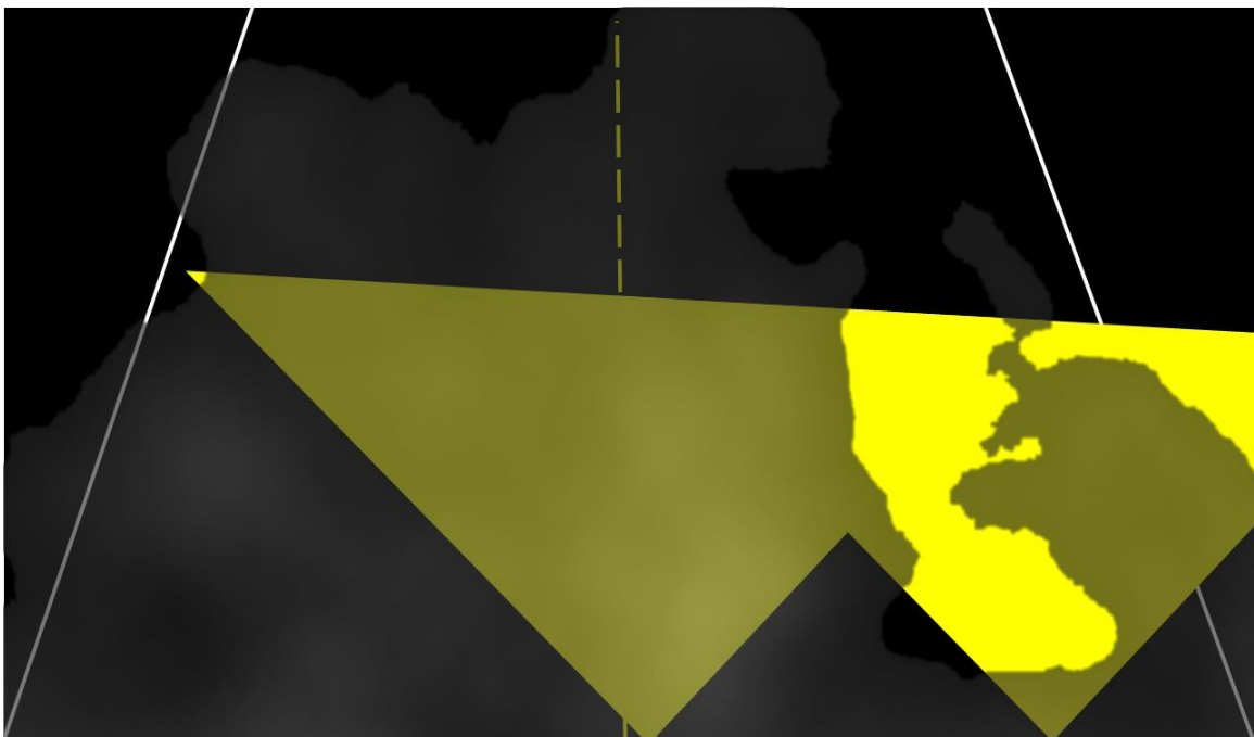
Figure 28. When fog is present it diffuses the light and reduces visibility. When there is a large amount of light present then the fog reflects a large portion of the light back. When we detect the large amount of reflected light then the system will switch to low beams and turn on the fog lights.
