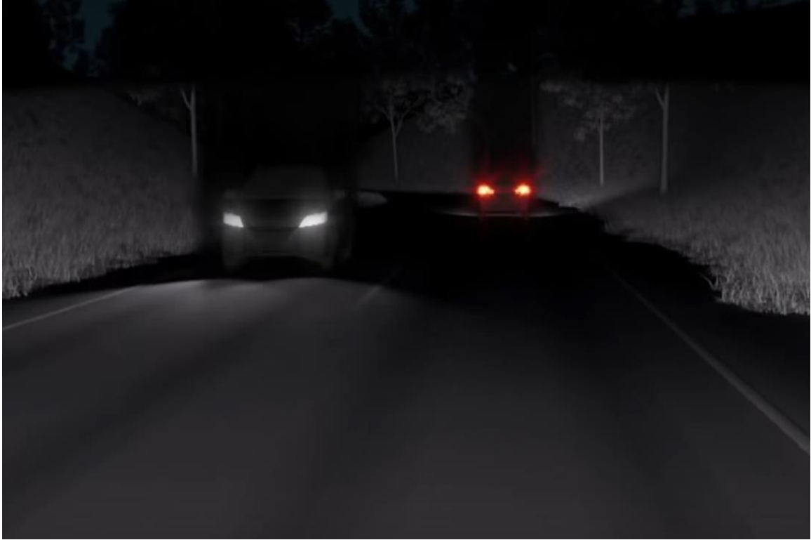
Figure 11. Toyota's LED array masking out a preceding car and an oncoming car while maintaining illumination of adjacent areas.
