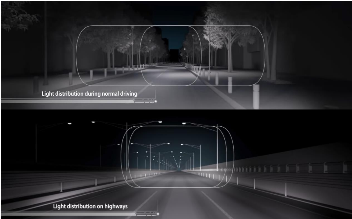
Figure 13. The car focuses the light in different areas to maximize the illumination based on the environment and driving situation.
